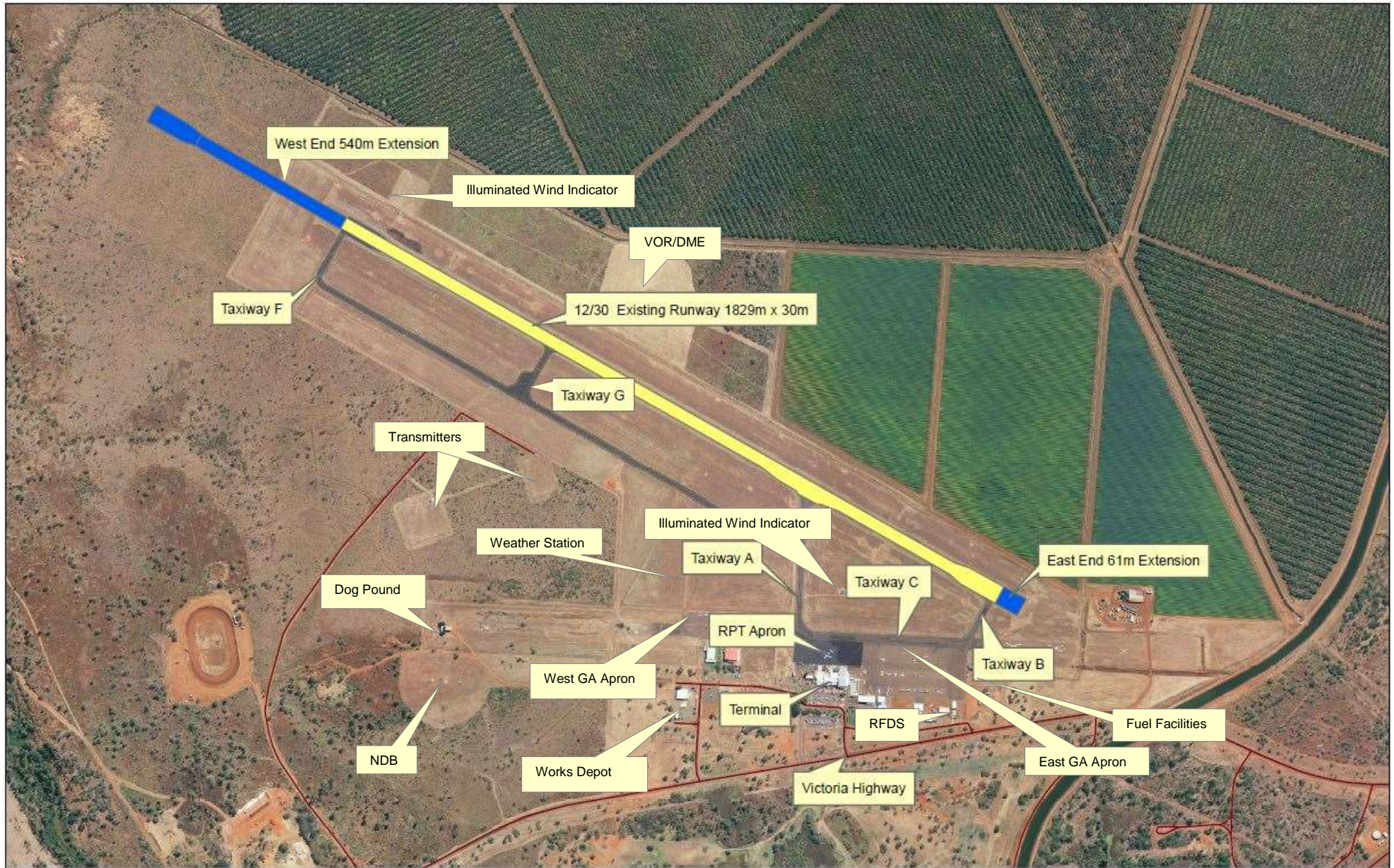
Figure 1 EKRA Existing Infrastructure and Proposed Runway Extension
