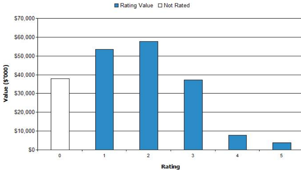
Figure 5.6: Sealed Roads and Drainage Asset Condition Profile
