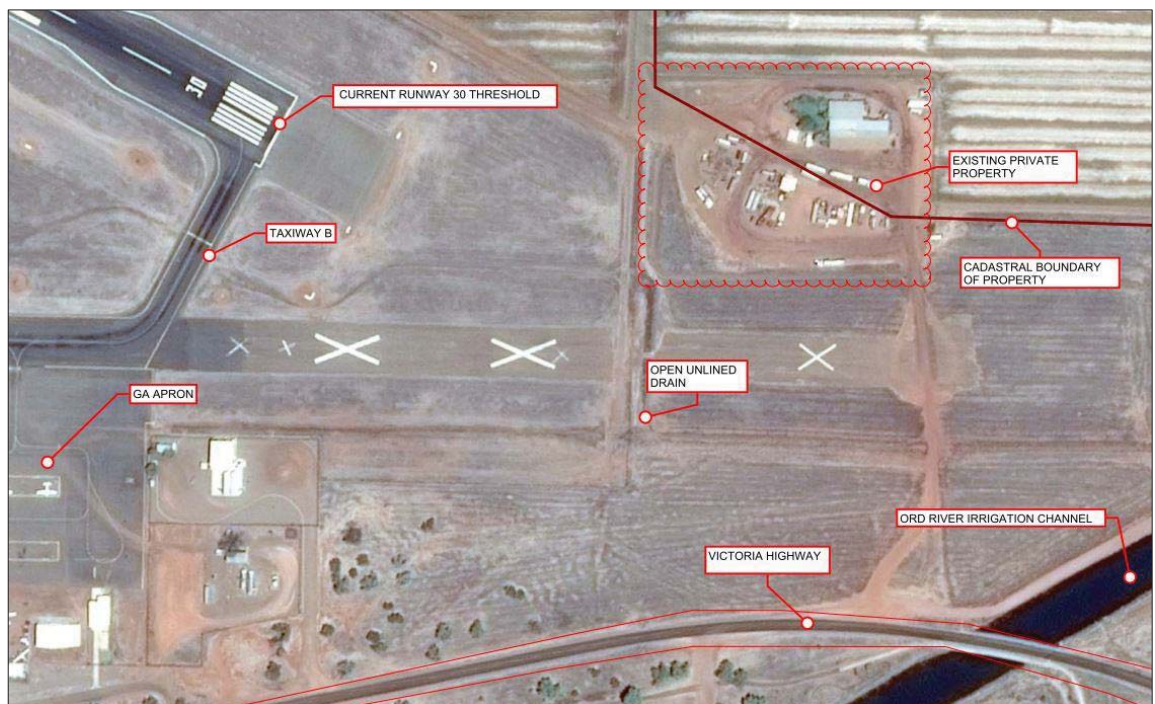
Figure 6 Eastern end extension constraints
