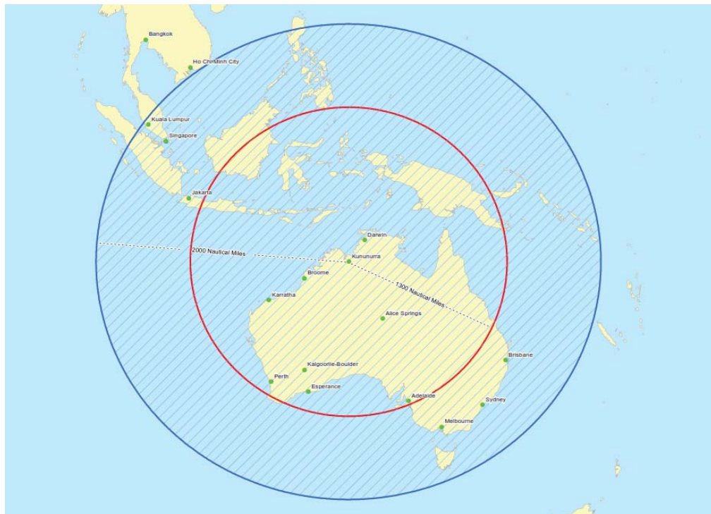
Figure 7 Range of existing Fokker 100 (red) vs proposed Boeing 737-800 (blue)
