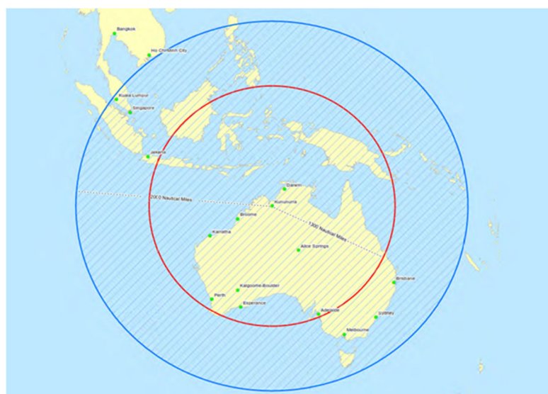
Figure 14: Range of existing Fokker 100 aircraft (red) vs proposed Boeing 737-800 (blue) from EKRA (GHD, 2016)
